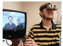
A set of goggles called JORDY functions like two high-definition television sets, with controls over color, contrast and magnification.
